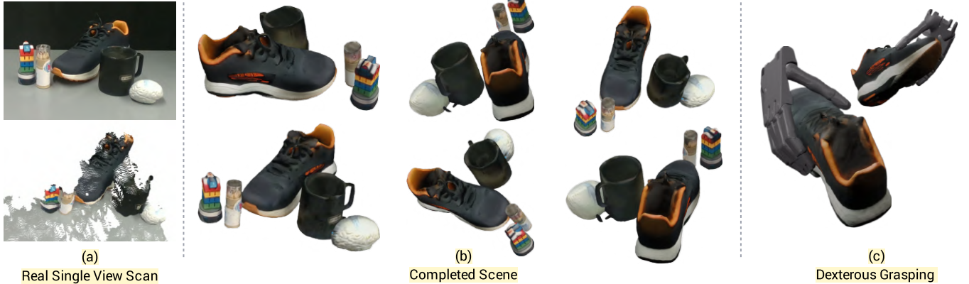
Fig. 1: (a) takes as input a single RGB-D image of a given scene, visualized here as a point cloud; (b) produces high-quality fully completed, accurately segmented object meshes in scenes with substantial occlusion and novel objects; and (c) enables downstream dexterous manipulation that requires accurate complete shape information.
