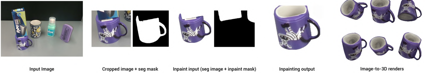
Fig. 12: Suboptimal inpainting outputs cascades to suboptimal image-to-3D generation.
